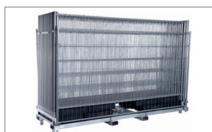
Transport and storage racks For 25, 29 or 30 Tempoform panels and associated blocks. Designed to be lifted using a forklift truck or a crane.
