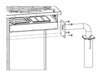
$5^{\circ}$ / Remove the burner assembly, fig.3 / 4:
