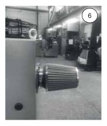
Once the collar is tight, the air filter is properly installed.
