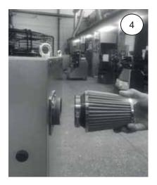
Place the filter on the air duct.
